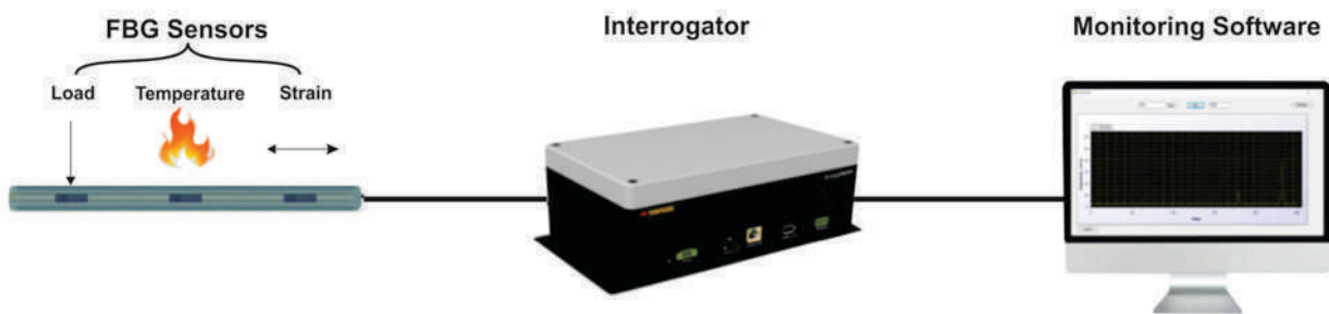
FBG sensor system configuration for Load/Temperature/Strain Sensing
