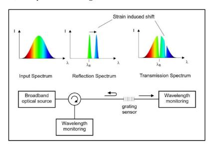
The reflected wavelength depends on the initial optical properties of the FBG that were embedded by the manufacturing process. In addition, the optical properties of the FBG depend linearly on the strain and the temperature. Change in one or every parameter will reflect back different wavelength to the reading unit. By determining the difference from the initial wavelength, it's possible to figure out the strain or the temperature within the FBG.
